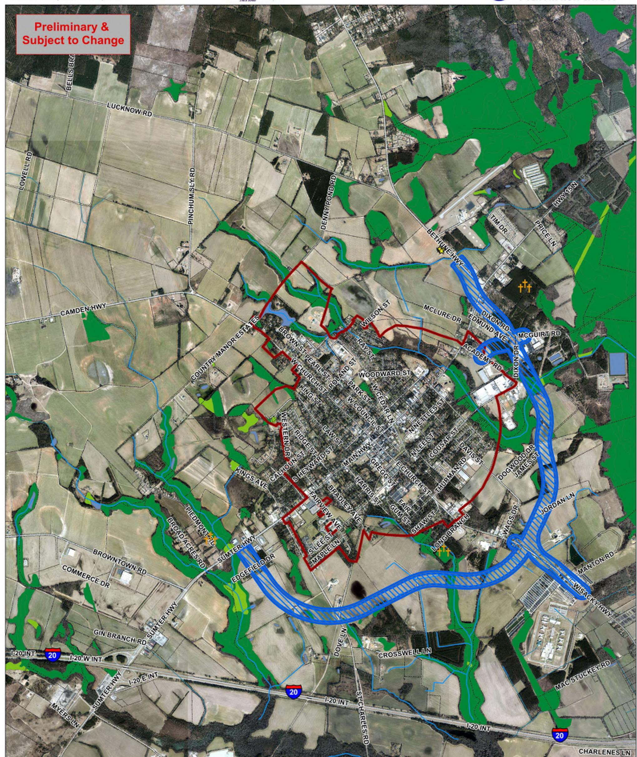
Note: The alternatives are still conceptual in design, so the corridors shown are 500 feet wide. Additional fieldwork, engineering, and public input will be used in the next phase of the project to identify the actual proposed width of the alternatives analyzed in the draft environmental impact statement.
