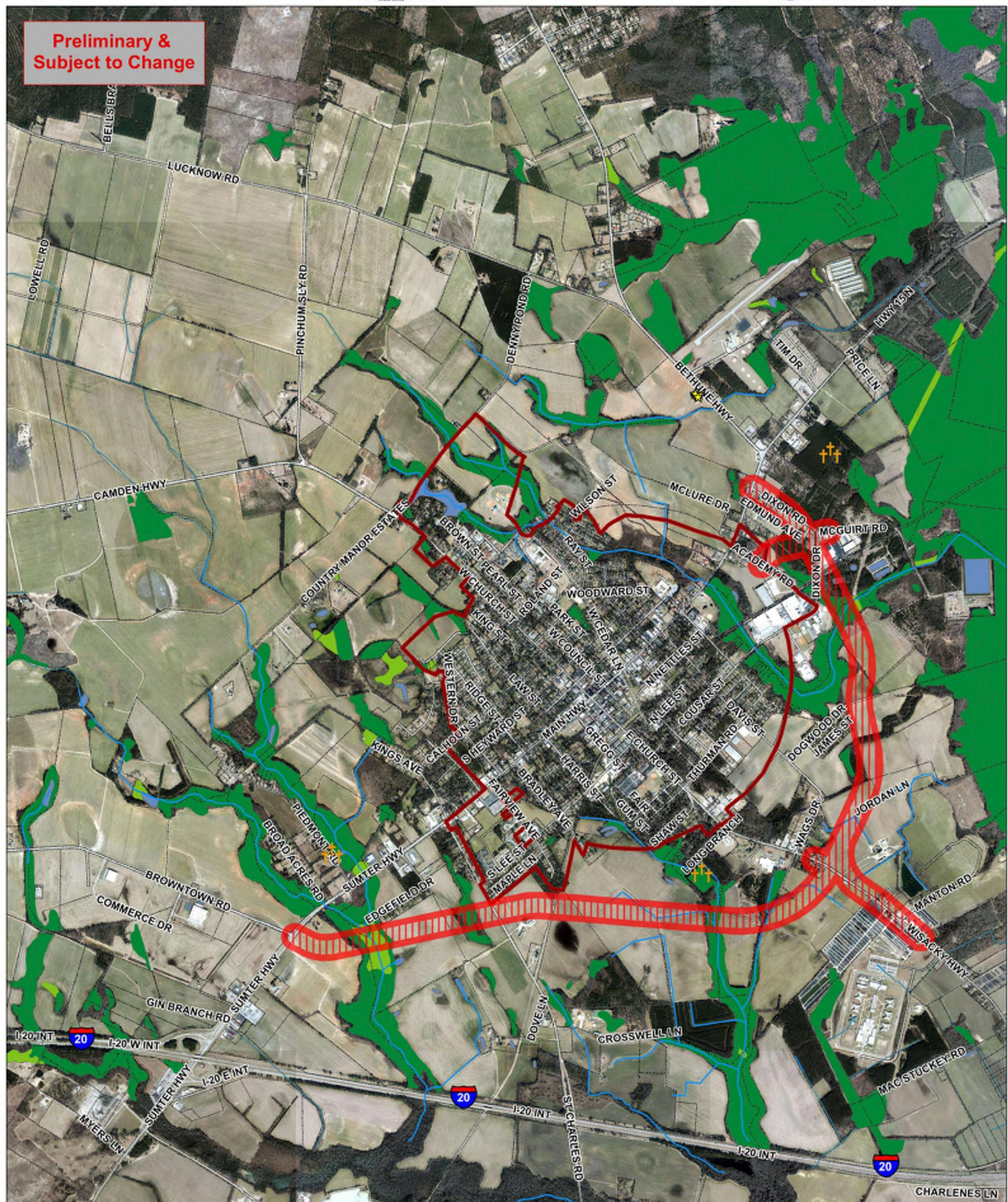
Note: The alternatives are still conceptual in design, so the corridors shown are 500 feet wide. Additional fieldwork, engineering, and public input will be used in the next phase of the project to identify the actual proposed width of the alternatives analyzed in the draft environmental impact statement.
