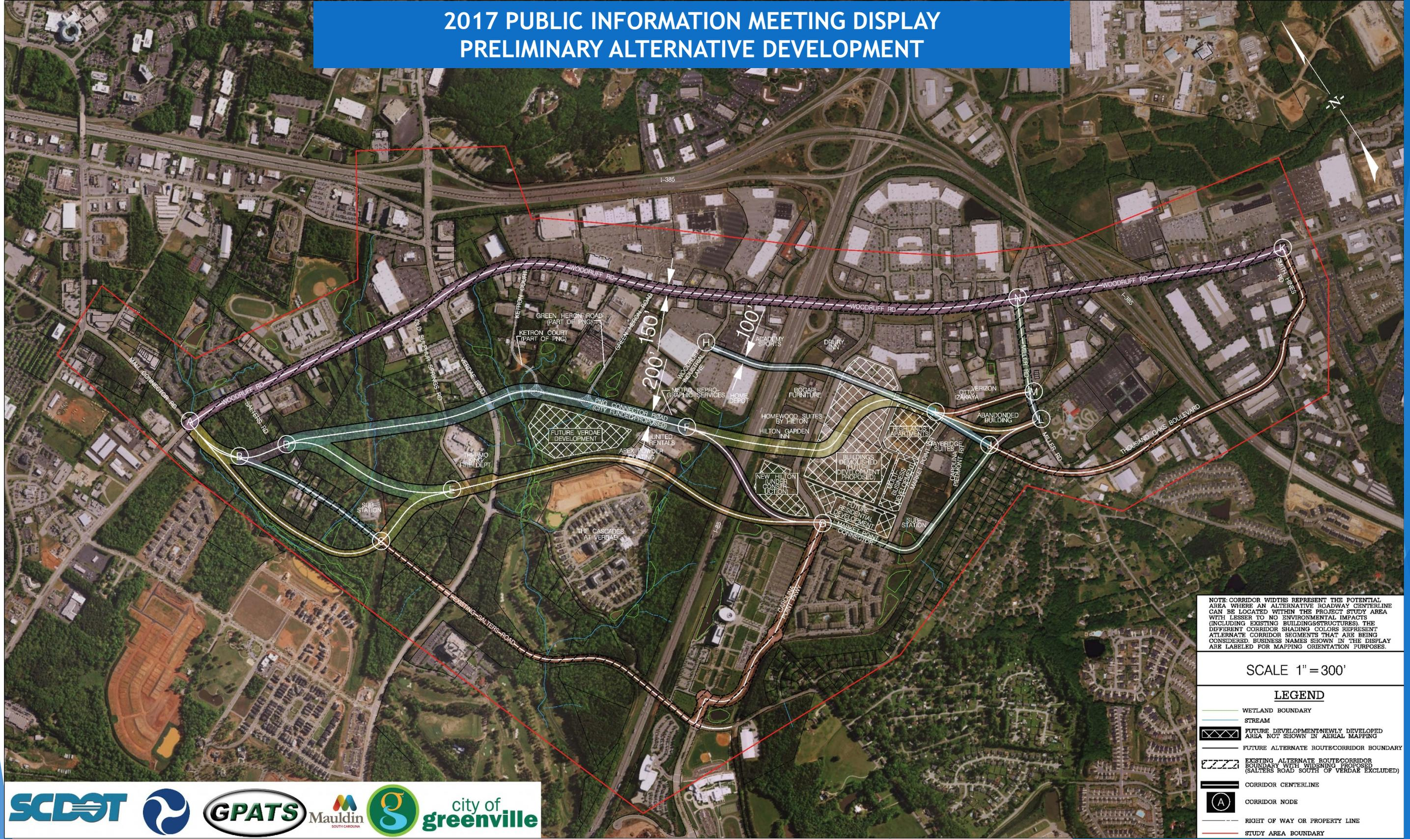
NOTE: CORRIDOR WIDTHS REPRESENT THE POTENTIAL AREA WHERE AN ALTERNATIVE ROADWAY CENTERLINE CAN BE LOCATED WITHIN THE PROJECT STUDY AREA WITH LESSER TO NO ENVIRONMENTAL IMPACTS (INCLUDING EXISTING BUILDINGS/STRUCTURES). THE DIFFERENT CORRIDOR SHADING COLORS REPRESENT ALTERNATE CORRIDOR SEGMENTS THAT ARE BEING CONSIDERED. BUSINESS NAMES SHOWN IN THE DISPLAY ARE LABELED FOR MAPPING ORIENTATION PURPOSES.
